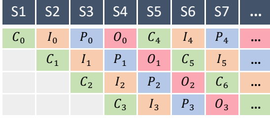
Figure 8: Cross-stacking view of CMU Groups. The S_i denotes the i -th MAU stage. The C_j , I_j , P_j , and O_j denote the four stages of CMU Group j listed in Table 2.
